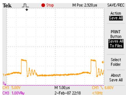
5.5V input with an 18mA load producing 28V DC output
