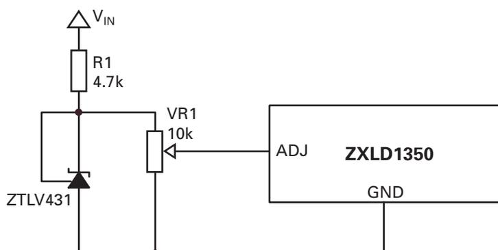
**Figure 5 Typical circuit of DC voltage dimming**
