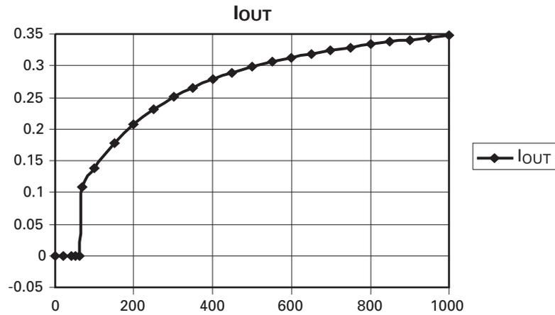
**Figure 6 Typical output current against pot resistance**
