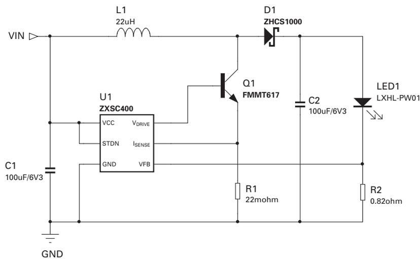
Figure 1 Schematic diagram
