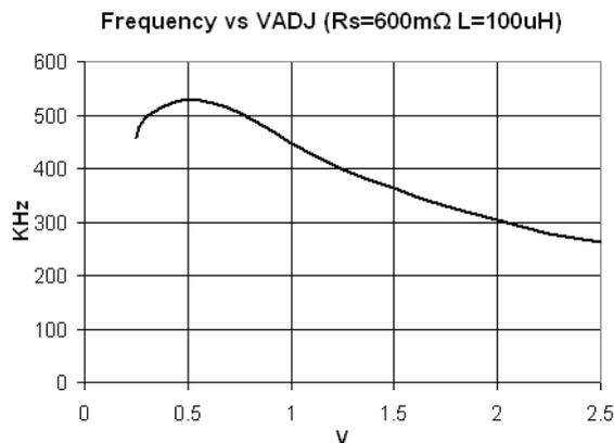
**Figure 4 Typical switching frequency versus ADJ voltage with  $R_S = 600\text{m}\Omega$ ,  $L=100\mu\text{H}$**
