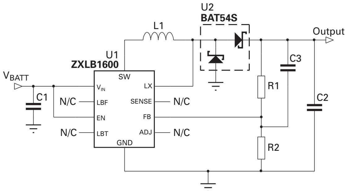
Figure 1 Schematic diagram
