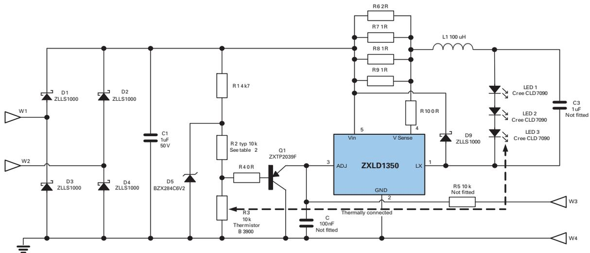
**Figure 2 Circuit diagram of ZXLD1350 MR16 lamp solution**
