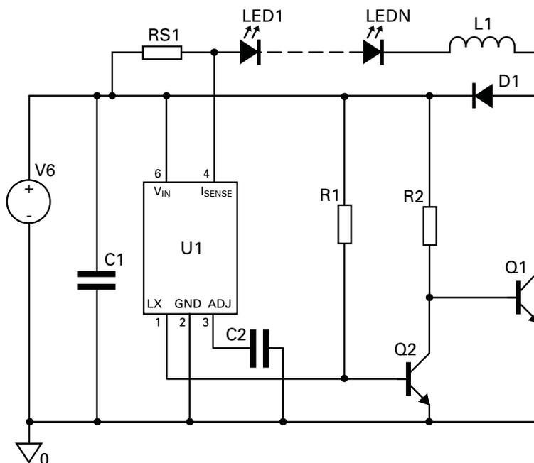
Figure 2 Schematic of 1A driver
