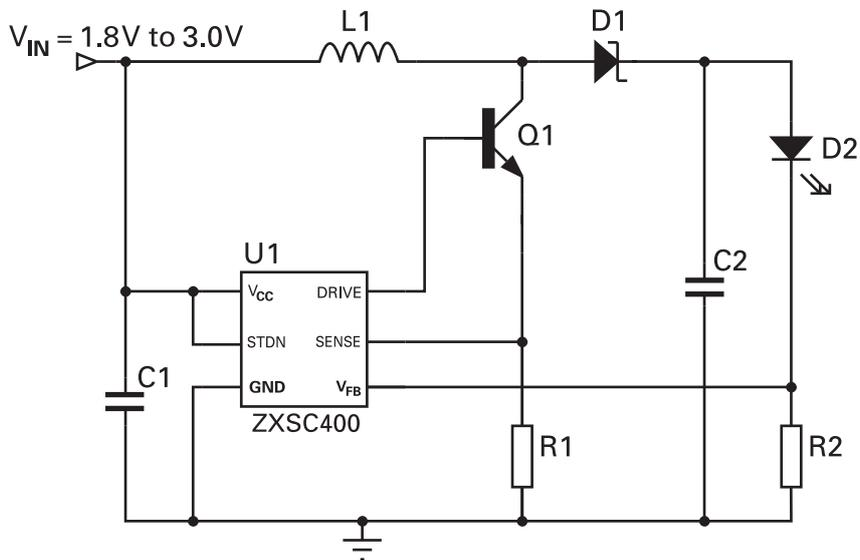
Figure 1 Schematic diagram
