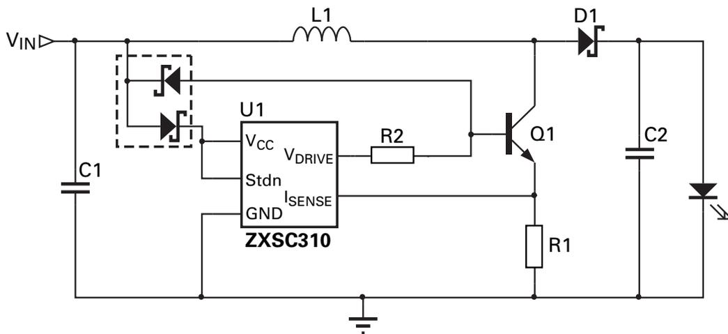
Figure 4 LED flashlight application without bootstrap
