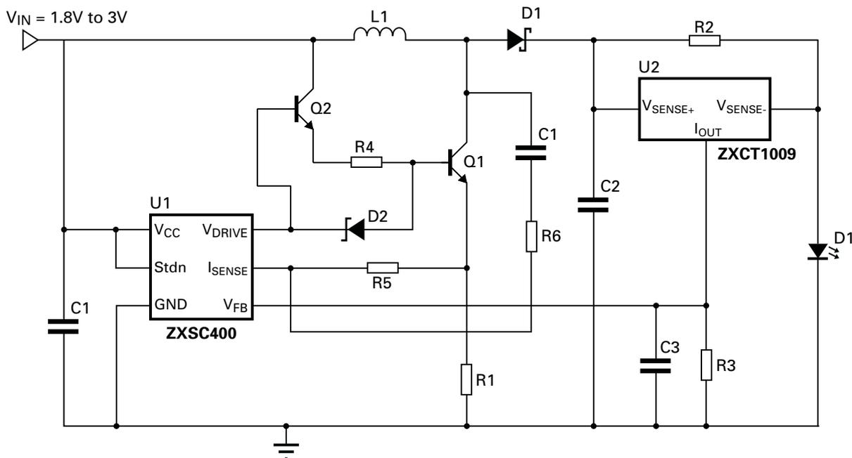
Figure 1 Schematic diagram
