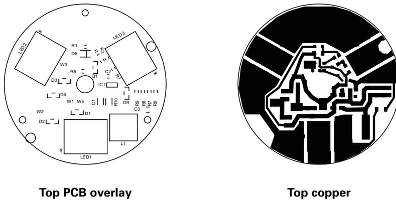
**Figure 5 Top PCB overlay and top copper**
