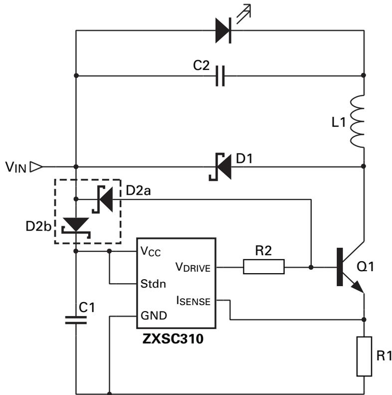
**Figure 5 Step down converter with reverse polarity protection**
