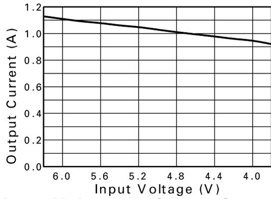
**Input Voltage vs Output Current**
