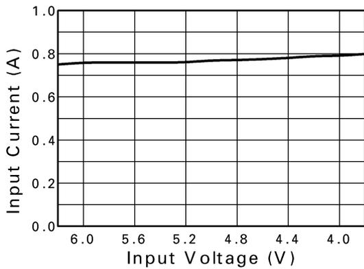
**Input Voltage vs Input Current**
