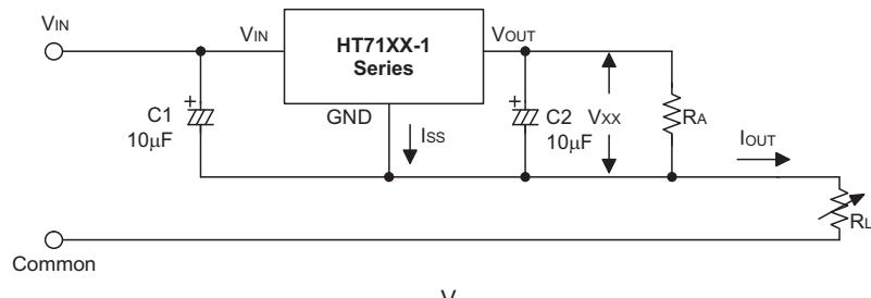
$$I_{OUT} = \frac{V_{xx}}{R_A} + I_{ss}$$
