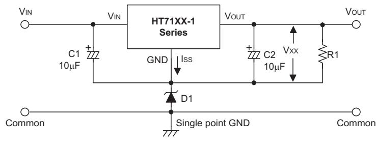
$$V_{OUT} = V_{xx} + V_{D1}$$
