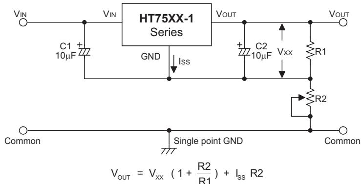
**Circuit for Increasing Output Voltage**
